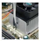
■Push the Front clip bar forwardand press down.
