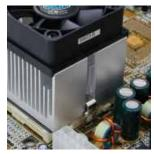
■ Hook The rear-endof the Clip Head on to Socket tip.
