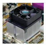
■Once in position. Pull bar back to secure cooler onto the socket.
